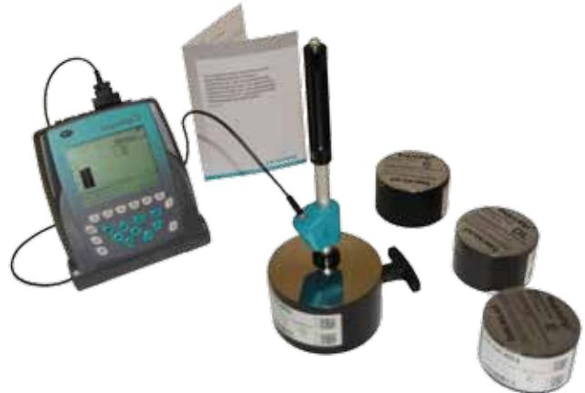
Equotip test blocks are delivered calibrated with the impact device that the customer uses to check his metal parts, e.g. in HLD, HLDL, HLE. This means that the calibrations are precise and are not based on conversions. Calibration certificates are issued by Proceq (factory calibration) or an accredited institute (national traceability), as per customer request.
