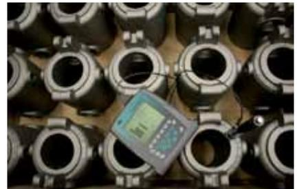
Standardized according to ASTM A956 and DIN 50156
