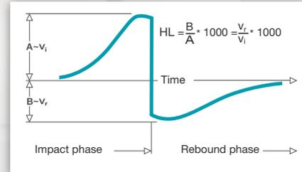
Velocities are measured using a permanent magnet in the impact body that generates an induction voltage in the coil which is precisely positioned in the impact device. The detected voltage is proportional to the velocity of the impact body. Signal processing is then providing the hardness reading.
