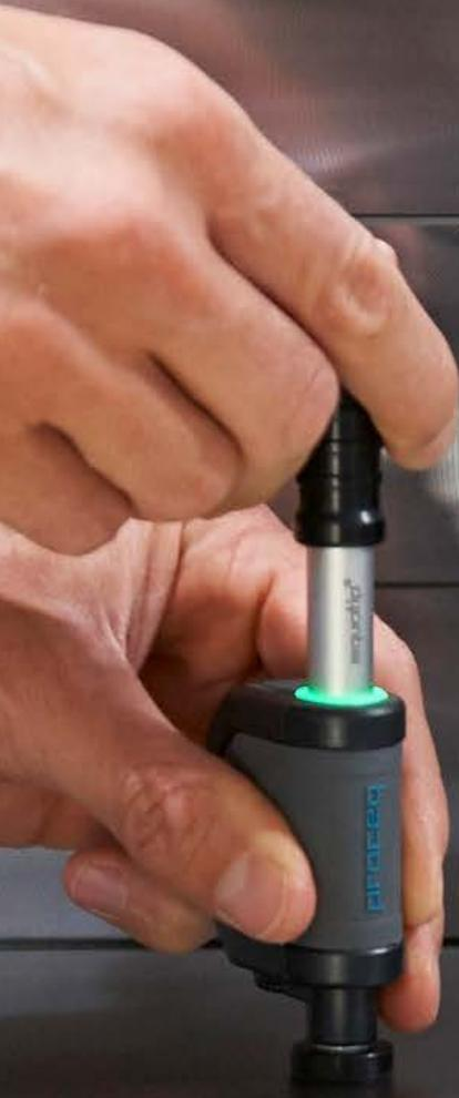
Leeb hardness principle is based on the dynamic (rebound) method. An impact body with a hard metal test tip is propelled by spring force against the surface of the test piece. Surface deformation takes place when the impact body hits the test surface, which results in loss of kinetic energy. This energy loss is detected by a comparison of velocities  $v_i$  and  $v_r$  when the impact body is at a precise distance from the surface for both the impact and rebound phase of the test, respectively.
