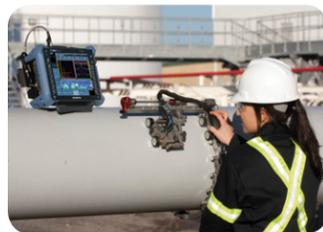
The OmniScan PA system with the HydroFORM scanner is designed to offer the best inspection solution for the detection of wall-thickness reductions resulting from corrosion, abrasion, and erosion. For this application, phased array ultrasound technology offers superior inspection speed, data point density, and detection.
