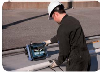
When coupled with the COBRA manual scanner, the OmniScan flaw detector is capable of inspecting pipes ranging from 0.84 inch OD to 4.5 inch OD. With its very slim design, this manual scanner is able to inspect pipes in areas with limited access.
