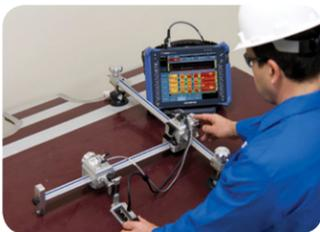
Olympus offers complete solutions for the inspection of carbon-fiber-reinforced polymer structures. These solutions are based on the OmniScan flaw detector, the GLIDER™ scanner, and dedicated probes and wedges designed for CFRP flat panel and radius inspection.
